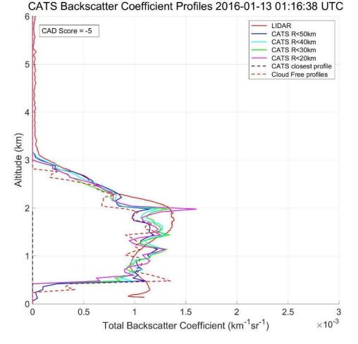
Figure 10. Total Backscatter Coefficient 1064nm profiles
